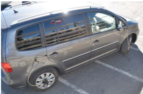
Fig1. VW Touran wheels instrumented for road testing.
