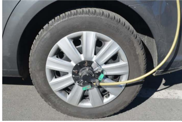
Figure 8: Thermocouple setup for recording data.
